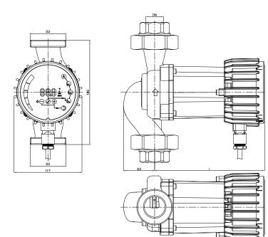
Flow Q up to 7,5 m³/h Pressure H up to 4 m Power 7 - 60 Watt Nominal pressure 10 bar
