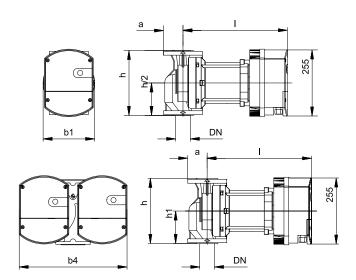
Flow Q up to 78 m³/h Pressure H up to 13 m Power 45 - 1600 Watt Nominal pressure PN6 or PN10
