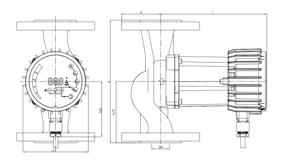
Flow Q up to 9 m³/h Pressure H up to 6 m Power 7 - 90 Watt Nominal pressure 10 bar
