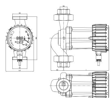
Flow Q up to 10 m<sup>3</sup>/h Pressure H up to 8 m Power 7 - 140 Watt Nominal pressure 10 bar
