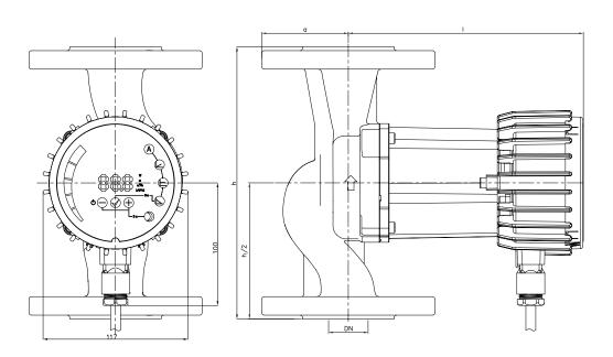
Flow Q up to 10 m<sup>3</sup>/h Pressure H up to 8 m Power 7 - 60 Watt Nominal pressure 10 bar
