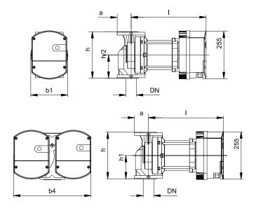
Flow Q up to 39 m<sup>3</sup>/h Pressure H up to 13 m Power 26 - 800 Watt Nominal pressure 6/10 bar
