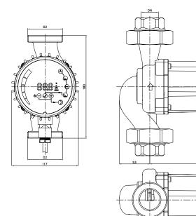
Flow Q up to 11 m<sup>3</sup>/h Pressure H up to 10 m Power 7 - 180 Watt Nominal pressure 10 bar
