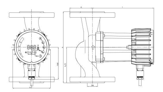
Flow Q up to 7,5 m³/h Pressure H up to 4 m Power 7 - 60 Watt Nominal pressure 10 bar
