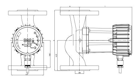
Flow Q up to 11 m<sup>3</sup>/h Pressure H up to 10 m Power 7 - 180 Watt Nominal pressure 10 bar
