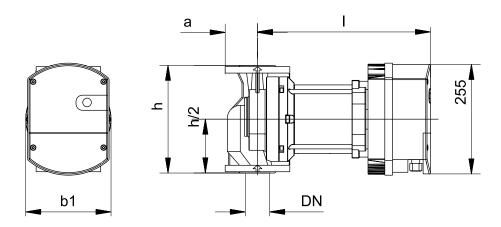
Flow Q up to 78 m³/h Pressure H up to 13 m Power 45 - 1600 Watt Nominal pressure PN6 or PN10
