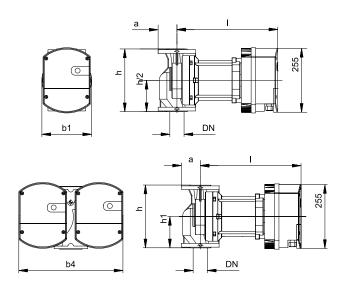
Flow Q up to 65 m³/h Pressure H up to 13 m Power 38 - 1100 Watt Nominal pressure 6/10 bar
