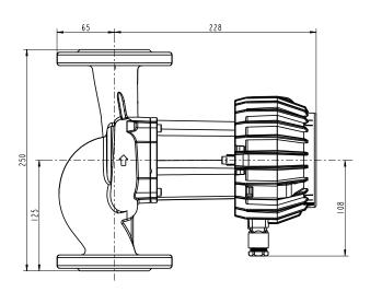
Flow Q up to 23 m<sup>3</sup>/h Pressure H up to 12 m Power 25 - 480 Watt Nominal pressure PN 6/10 bar
