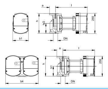
Flow Q up to 39 m³/h Pressure H up to 13 m Power 26 - 800 Watt Nominal pressure 6/10 bar
