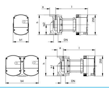
Flow Q up to 25 m³/h Pressure H up to 13 m Power 20 - 500 Watt Nominal pressure 6/10 bar
