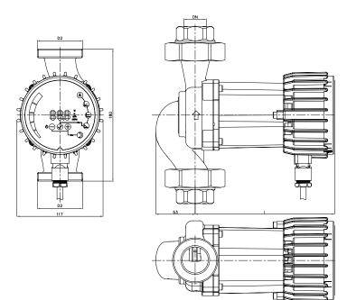
Flow Q up to 9 m³/h Pressure H up to 6 m Power 7 - 90 Watt Nominal pressure 10 bar
