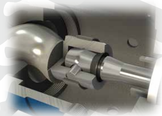
Cross Section of Pin Joint in the Rotor Head
